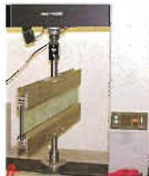
National Technical Systems, a certified laboratory, tested the Wedge-Lock™ Door Rail System at a temperature range from -10° to 150° F, with 1000 pounds of tension load applied. No evidence of movement was detected at any temperature. At an ambient temperature of 75° F, in a "Pull to Failure Test", 6950 pounds of tension was required before any creep (no failure) was detected.
