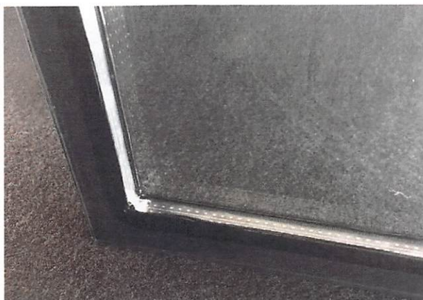
Figure 4: An Example of Primary Sealant Infringement
