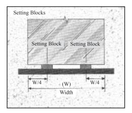
glazing. If setting block shims are required, they must be located under the setting blocks and have a durometer rating equal to or greater than that of the setting blocks. Failure to properly design and locate setting blocks can cause point pressures, bending stress, or glass-to-metal contact resulting in glass breakage or ponding of water, a primary cause of seal failure in insulating glass units.
