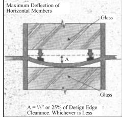
Anchors and expansion joints should be designed so that loads are not applied to the glass framing due to the thermal or mechanical movement of the structure. For a stick system, there should be a vertical expansion joint at every floor and preferably at a horizontal support member. Vertical expansion joints should be at glass corners and never placed along an edge of insulating glass.
