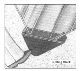
or grinding. Corner edge damage can also occur when glass is rotated on a hard surface prior to glazing. It is recommended that a "rolling block" be used by glaziers to rotate the unit. The rolling block minimizes the chance of damage to the corner of the glass by distributing the glass weight along the edges rather than concentrating it at the corner.
